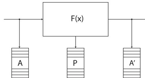
Figure 2: An overview of the SAFE data collection architecture, where  $A$  represents the audio features captured before the effect is applied,  $A'$  represents the features captured after the effect is applied, and  $P$  represents the parameter vector.
